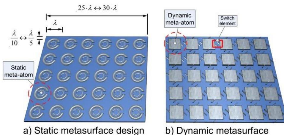
Fig. 9 Example of static and dynamic meta-surfaces made of meta-atoms. From [23]
