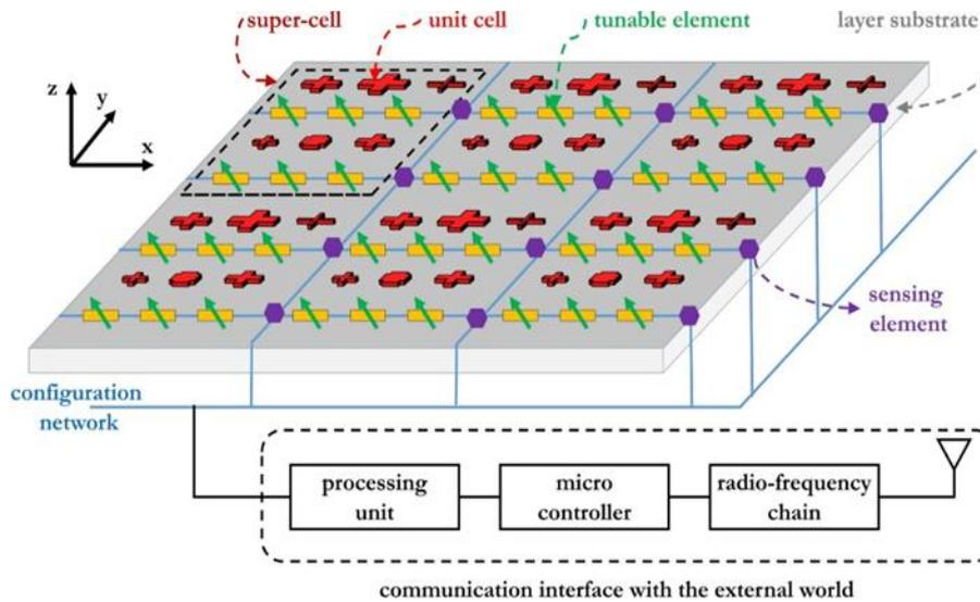
Fig. 10 Conceptual structure of a reconfigurable intelligent surface. From [14]
