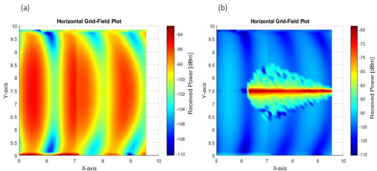
Fig. 14 Coverage map of the receiver grid at the height of 4.2m: (a) Room without windows and hole, (b) Room with windows and hole
