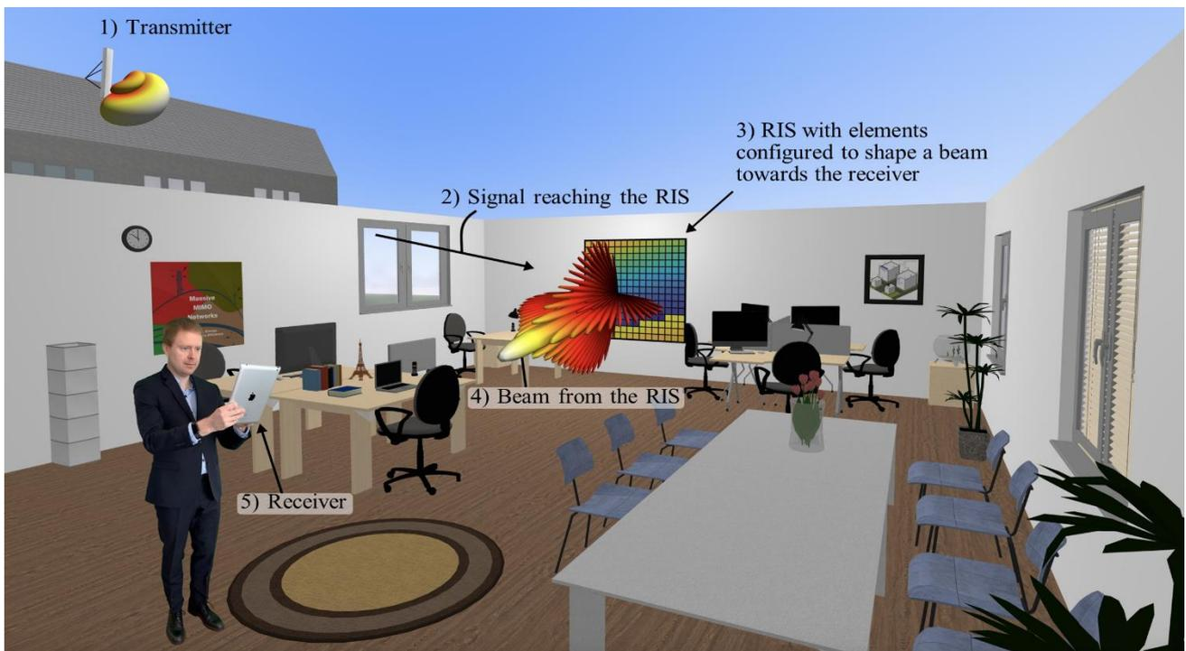
Fig. 7 A typical use case of an RIS, where it receives a signal from the transmitter and re-radiates it focused towards the receiver. To focus the beam in the right direction, the RIS must be configured properly. From [18]
