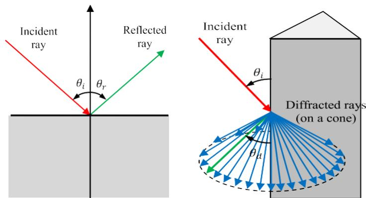
Fig. 5 The reflected ray (left) from a planar interface between two different mediums and the diffracted rays (right) from an edge. Note that there is only one single reflected ray but a continuum of diffracted rays (on a cone). Adapted from [11]
