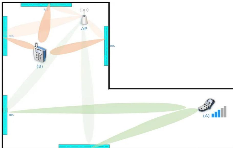
Fig. 6 The RISs can be optimized to improve signal strength even in NLOS case. From [17]
