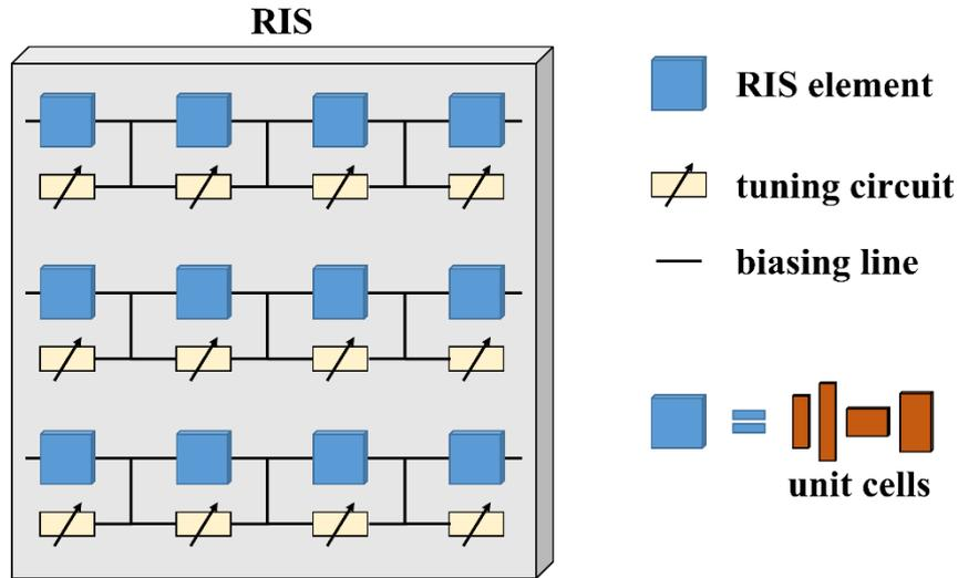
Fig. 8 Conceptual architecture of a reconfigurable intelligent surface. Adapted from [20]
