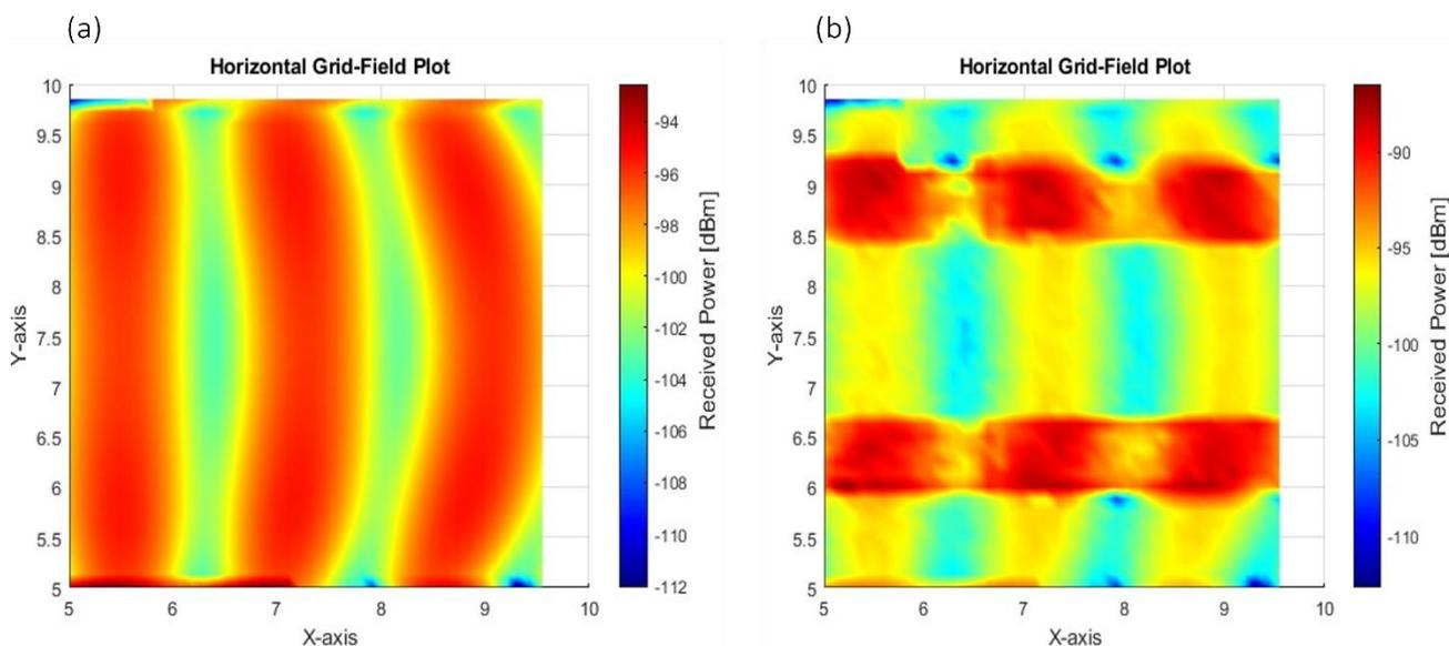
Fig. 15 Coverage map of the receiver grid at the height of 5.8m: (a) Room without windows and hole, (b) Room with windows and hole
