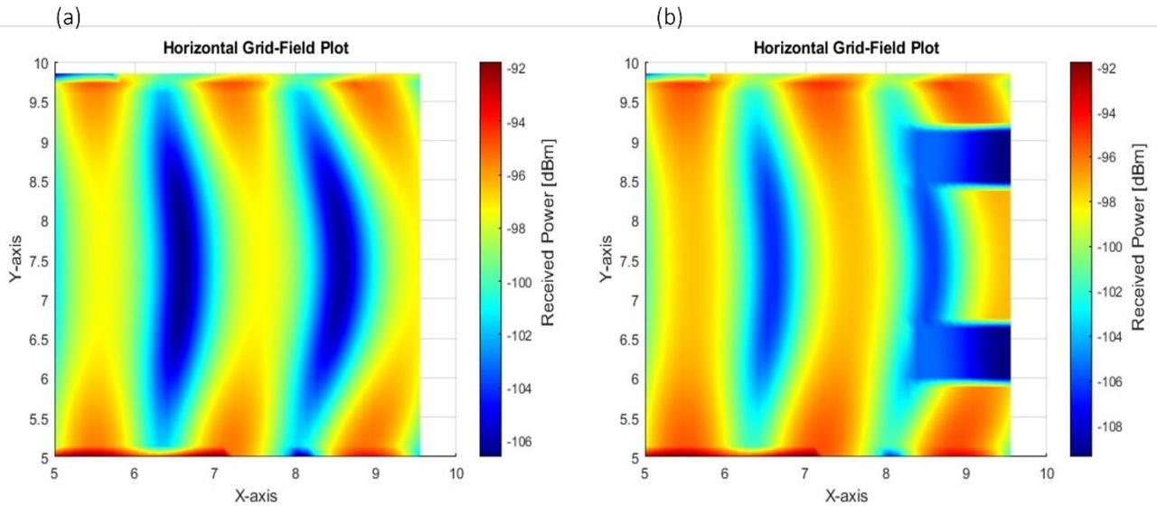
Fig. 16 Coverage map of receiver grid at the height of 7.0m: (a) Room without windows and hole, (b) Room with windows and hole
