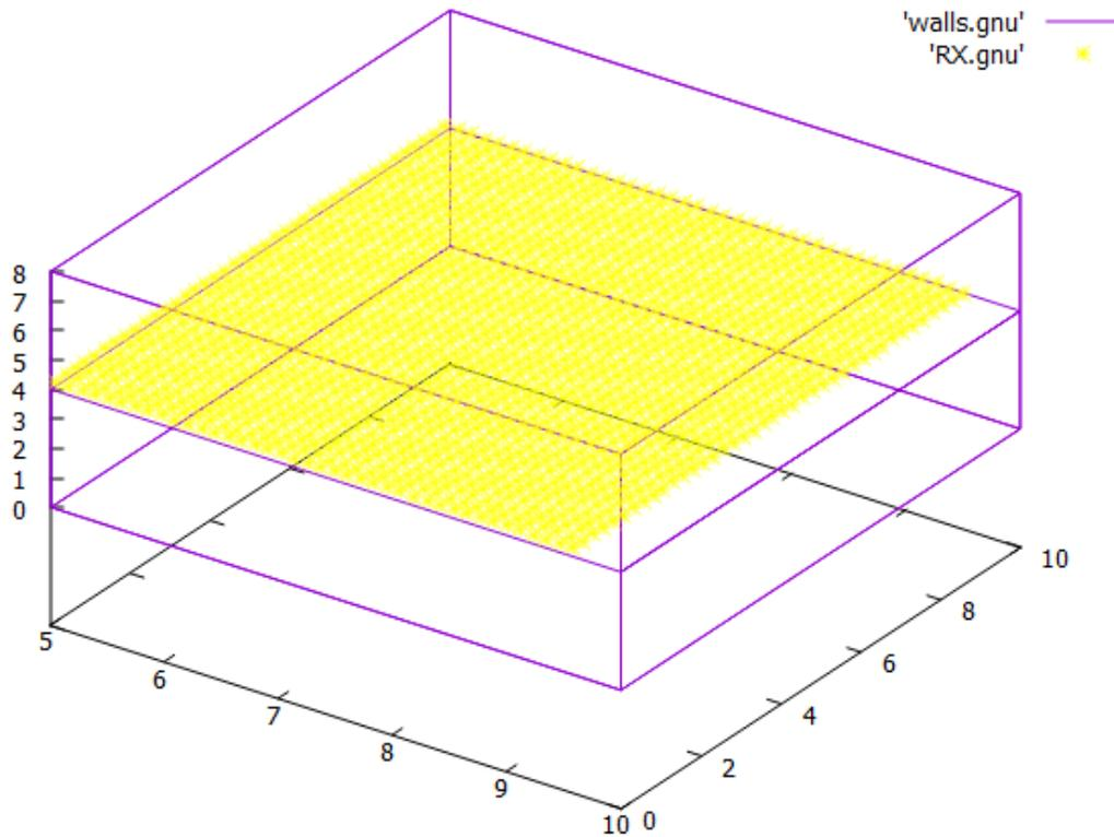
Fig. 12 3D plot of the building with grid of receivers at 4.2m on second floors room
