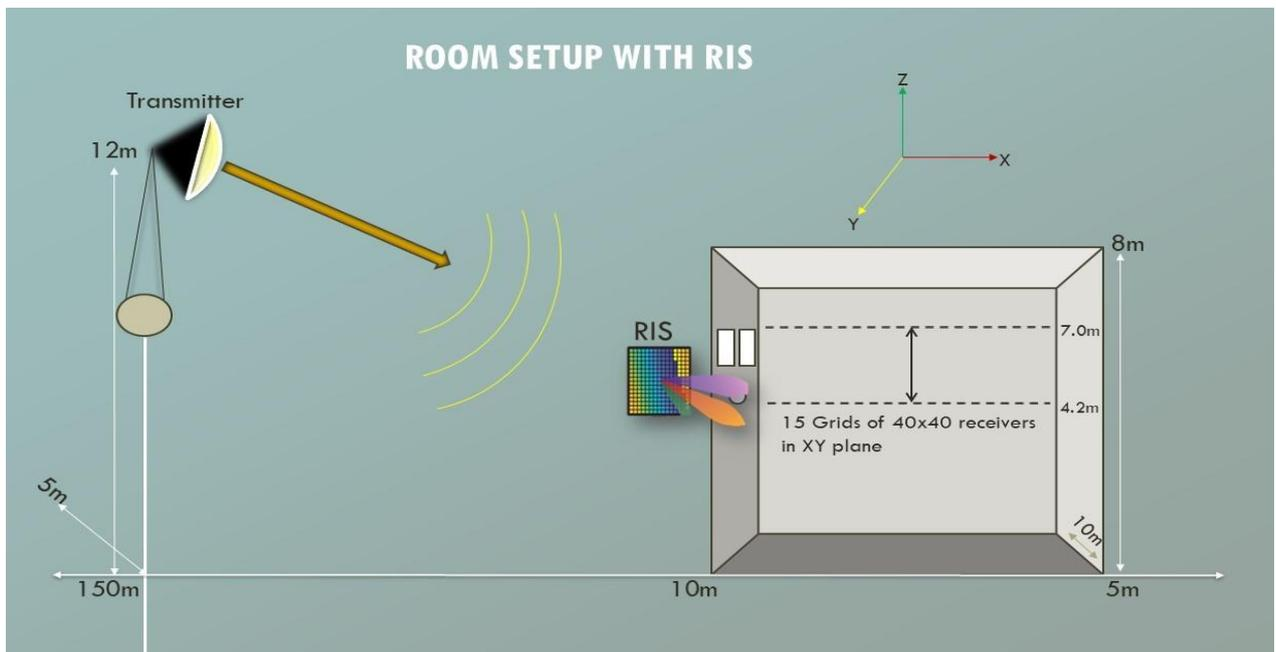
Fig. 4 An enhanced setup incorporating Reconfigurable Intelligent Surface
