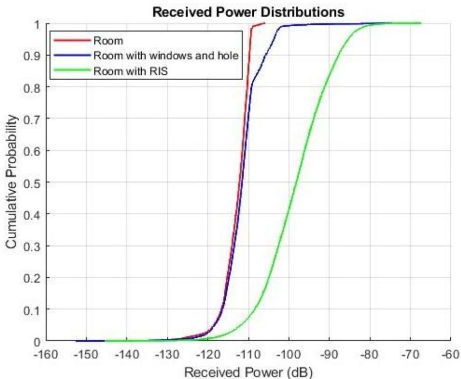
Fig. 20 CDF for three cases: Simple room, room with windows and hole, room with RIS
