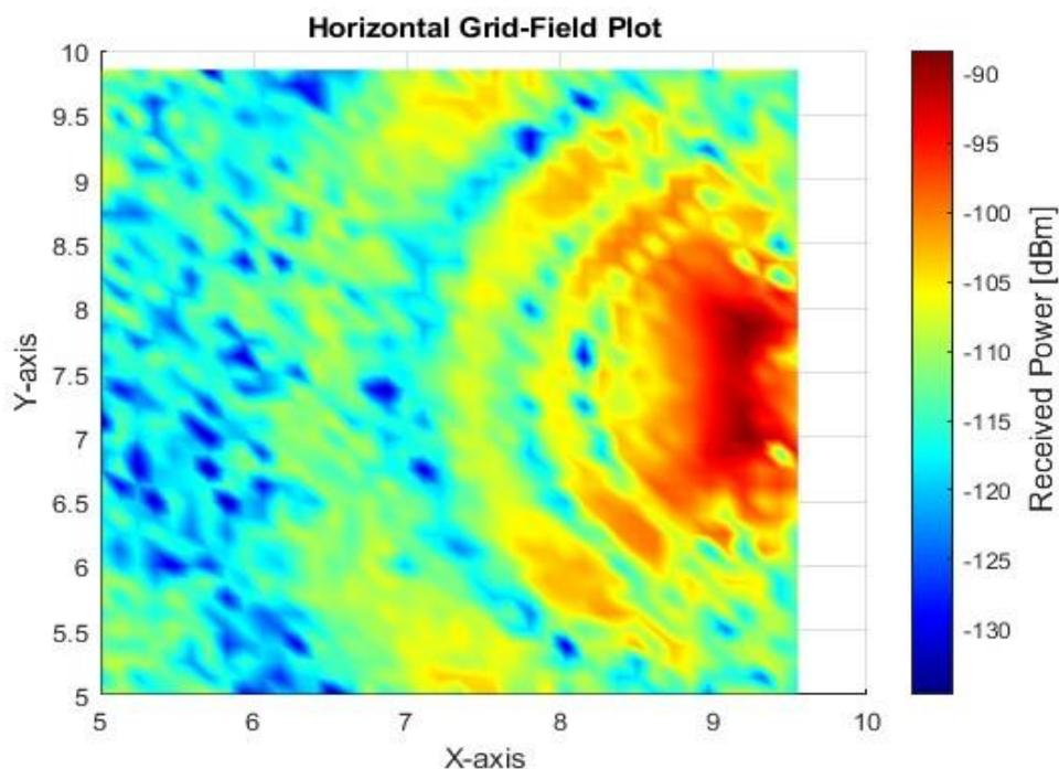
Fig. 19 Coverage map of the receiver grid at 4.2m with RIS
