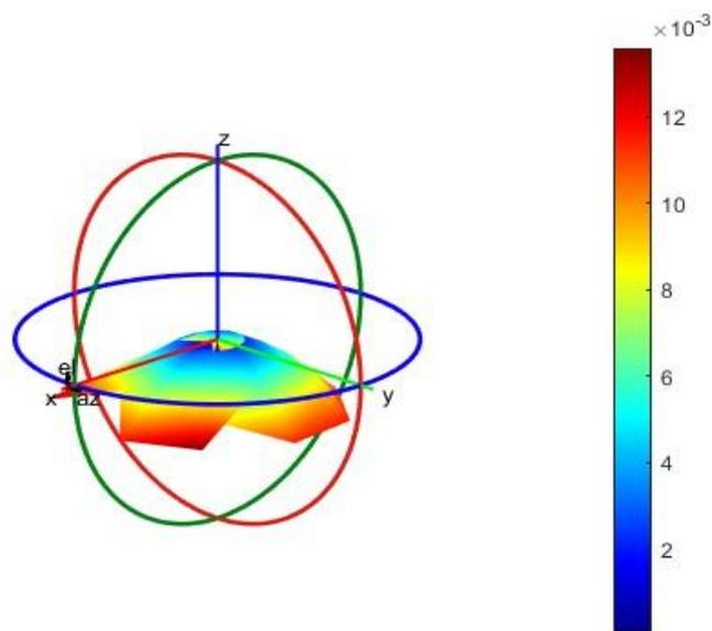
Fig. 18 Simulated re-radiation pattern of the RIS
