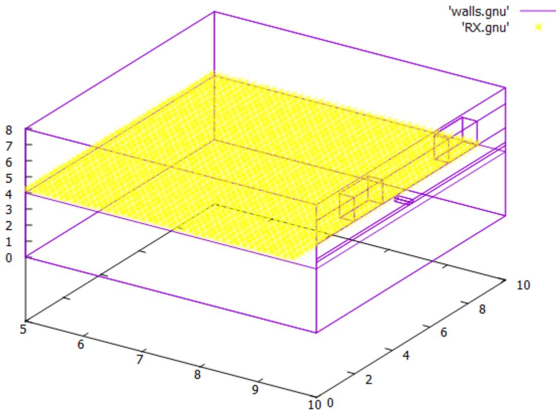
Fig. 13 3D plot of simulation environment with walls, windows, hole and their frames that contribute to diffraction effects.
