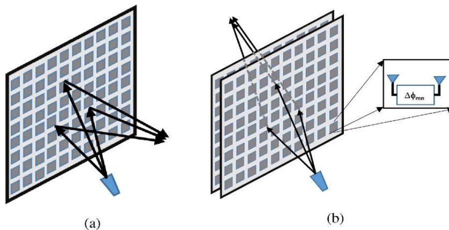
Fig. 2 Illustration of (a) reflective metasurface and (b) transmissive metasurface. From [5]
