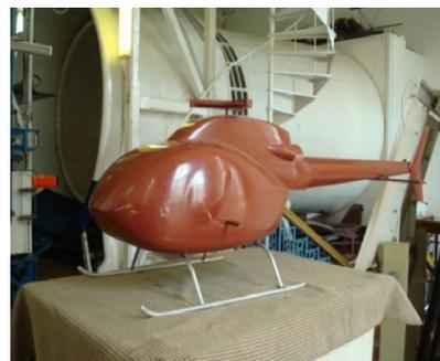
(b) Wind tunnel model of the AKTAY helicopter fuselage [32].
