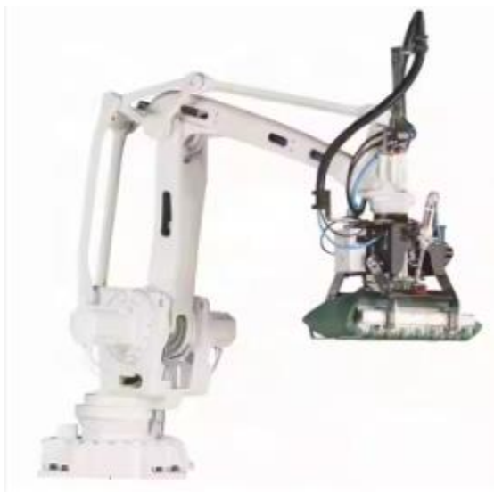
Figura 8: IRB 460 Palletizing Robot 4 Axis Industrial Robot Arm High Speed Palletizer With Gripper
