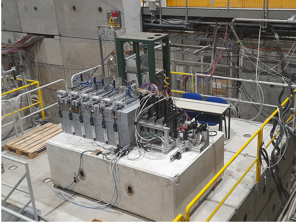
Figure 2.8: Picture of the test beam setup. The SciFi detector is on the right, and the backward section includes the US stations.
