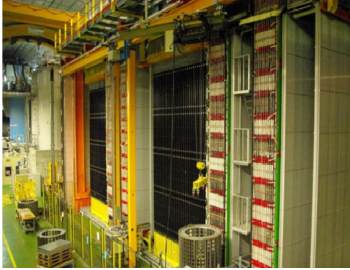
Figure 1.13: OPERA experiment in Gran Sasso Laboratories, it can be seen the two modules of the experiments, made by 27 walls, composed by 75000 bricks of lead covered by photographic films.
