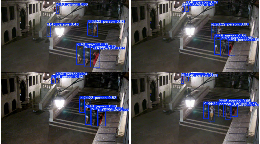
Figure 4.6: Example of pre-trained YOLO tracking inference on four frames of a video shot at night time. The model only detect the most illuminated people on the foreground, but surprisingly keep them tracked with the same ID. The images are 6 frames (2 seconds) apart.
