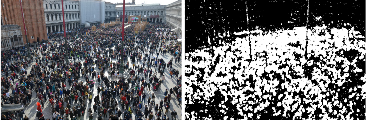
Figure 4.22: The image from the dataset with the largest number of people (3975) and the corresponding U-Net inference. It is clear that, even if the U-Net output is acceptable and generally correct, most of the circles (i.e., detected people) are considered as a single contour and thus counted only once. However if the location variables (distance from the camera, zoom level, etc) are known, the number of white pixels can be associated to the number of people.
