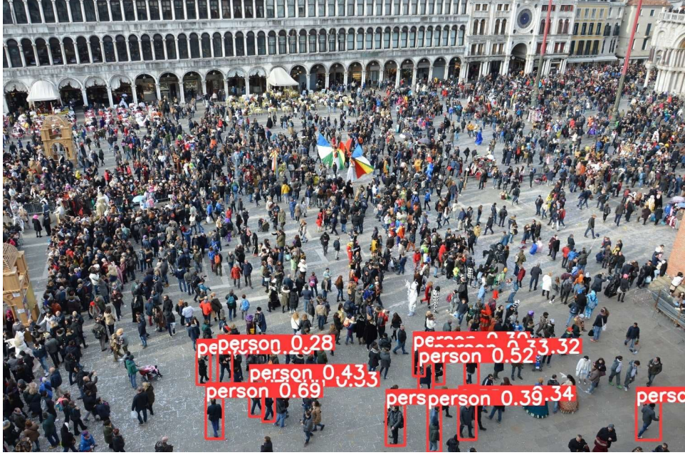
Figure 4.4: Example of pre-trained YOLO detection inference on an image of the dataset. It is clearly visible how the model works only in low crowd density conditions.
