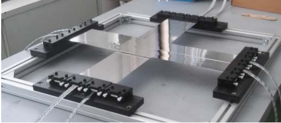
Figure 3.9: Picture of the scintillator bar array tested at n_TOF-EAR2 in 2023.
