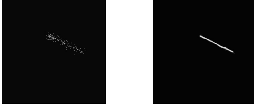
(A) Aberrated track on the sensor. (B) Predicted track segment.
