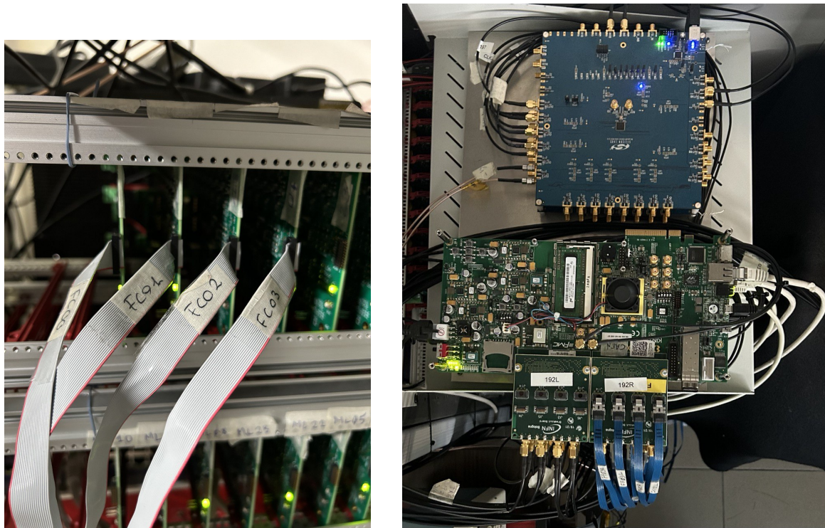
Figure 3.25: Connections of the Adapter Boards with the Master Logic (left) and of the ALCOR chip with the FPGA and clock system (right)
