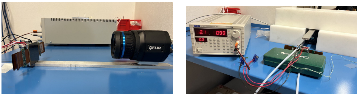
Figure 3.19: Photon detection unit sensors aligned with the FLIR thermal camera (left) and the stabilized setup of the test (right) drawing attention to the power supply connected to the Peltier cells and the water circulating pipes.
