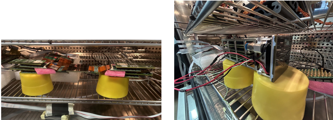
Figure 3.6: Set-up of the NTC functionality test inside the MEMMERT climatic chamber for SiPM S1375-1, S1375-2, S1375-3, S1375-5 (left) and S1350-1, S1350-2, S1350-3, and S1350-4 inside the mini crate (right).
