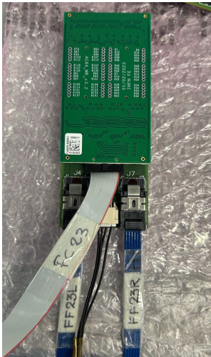
Figure 3.22: Connections of the single ALCOR and adapter boards.
