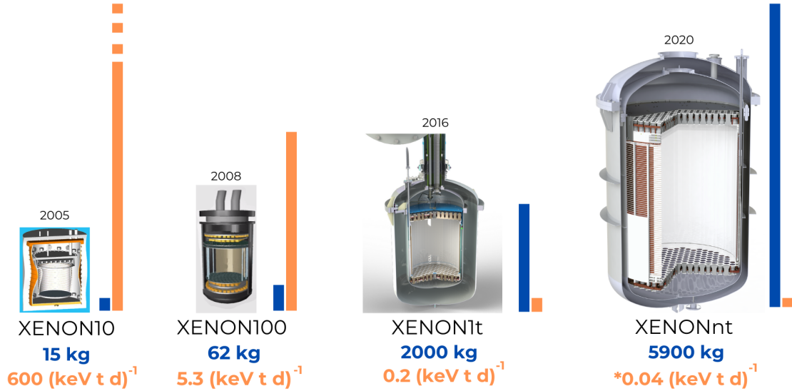
Figure 2.1: Overview of the XENON program detectors, showcasing the TPCs of varying dimensions and with the construction year noted. Displayed in blue are the active LXe masses within the TPCs. The orange indicator represents the low-energy (below 20 keV) ER background level measured in each experiment. Figure re-adapted from [10].
