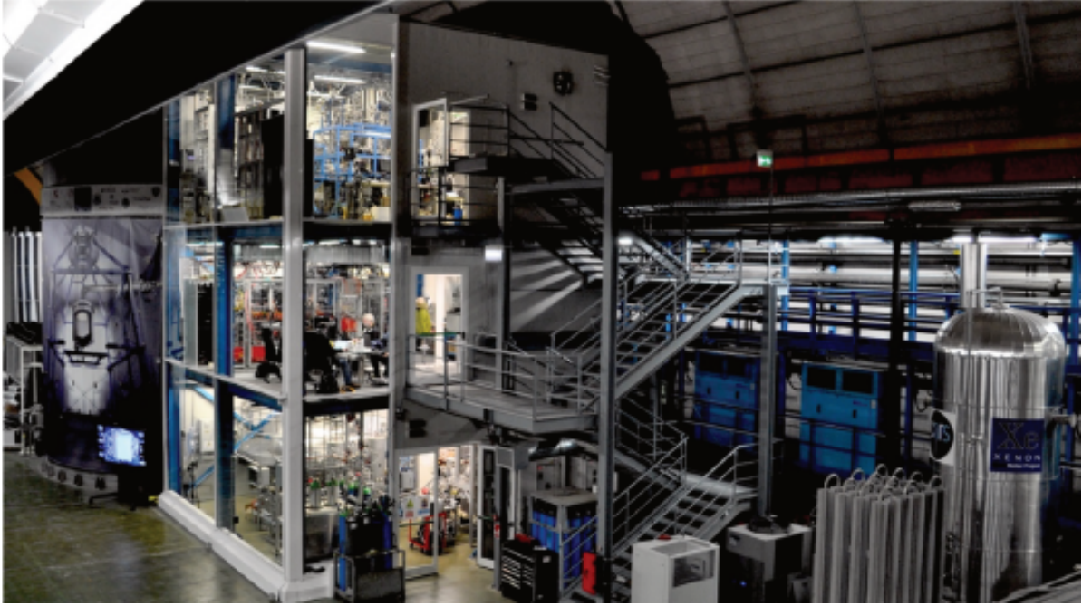
Figure 2.2: A view of the XENONnT experiment located in hall B at LNGS. Prominently featured in the background is the water tank, serving both as a passive shield and an active water Cherenkov Muon and Neutron Veto. At the heart of the water tank, the TPC stands as depicted on the overlaying poster. In the foreground, the service building is visible, housing the various subsystems of the experiment including cryogenics, Xe purification, distillation, recovery, and the DAQ system.
