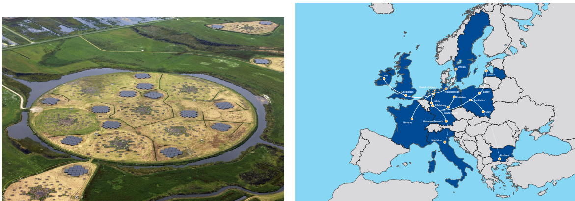
Figure 4.1: Left: aerial photograph of the “Superterp”, in the central part of the LOFAR core, showing the distribution of both HBA and LBA antennas. From van Haarlem et al. (2013) . Right: international distribution of the LOFAR stations across Europe, considering also the station under construction (and planned). Credits: ASTRON, https://www.astron.nl/telescopes/lofar/ .
