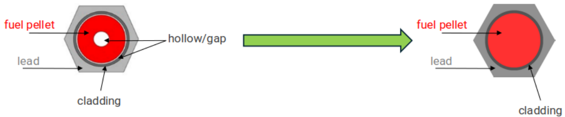
Figure 4.2: Simplified Fuel pin cell model.
