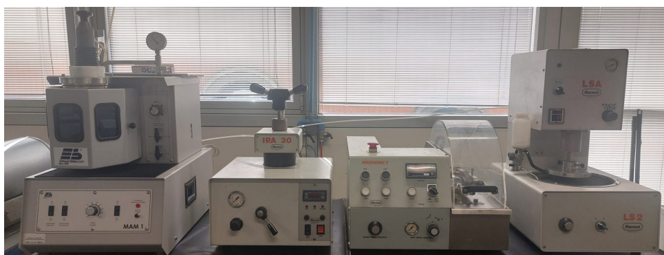
Figure 3.2: From left to right: Arc Melter, Automatic Mounting Press, Cutting Machine, Polisher.
