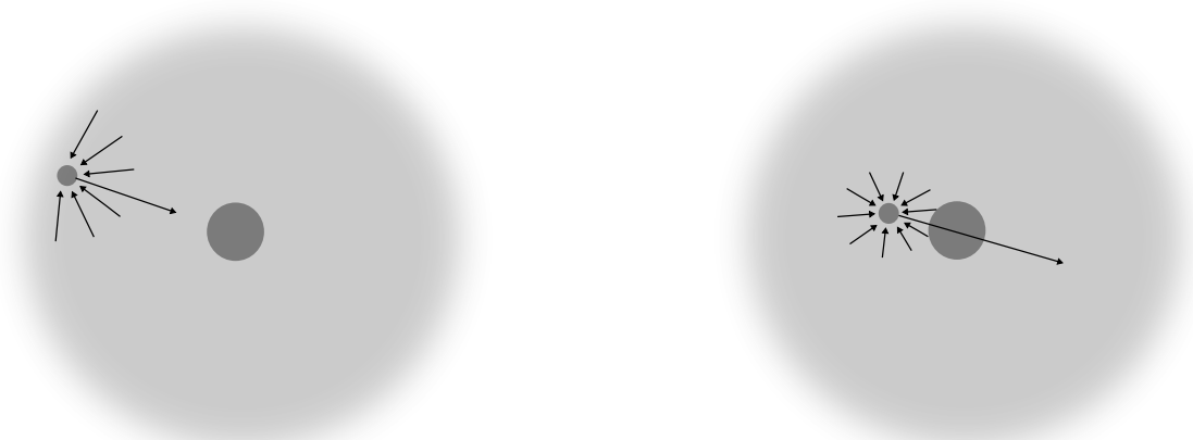
Figure 1.2: Left: The nucleus exerts a strong attractive force on an electron near the atom's surface, while the other electrons apply weak repulsive forces. The net impact of these repulsive forces is significant. Right: The nucleus exerts a very strong attractive force on an electron close to the atom's center, while the other electrons apply weak repulsive forces. (The figure was redrawn: it is based on Fig. 9-8 of [9])
