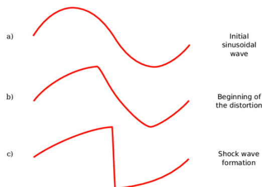
Figure 17: The figure shows the formation of a shock from an initial sinusoidal wave. Adapted from Pozzi (2014)
