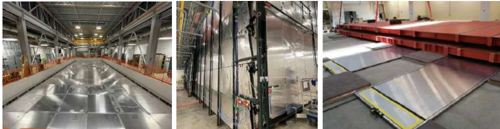
Figure 4.2: Pictures of the (Left) Top CRT before the overburden deployment on top, (Center) Side CRT, and (Right) Bottom CRT on the ground pit of the ICARUS cryostat.
