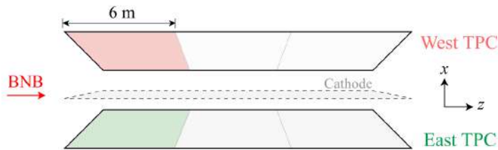
Figure 3.11: View from the top of the West ICARUS T300 module. The front-facing sections of the TPCs are shown.
