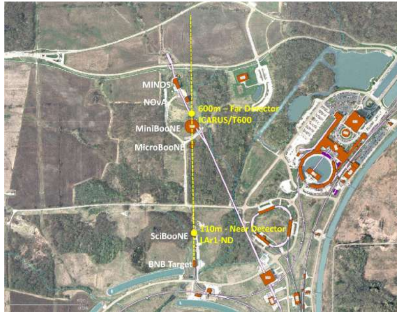
Figure 2.1: Approximate locations of the detectors superimposed on an aerial view of the Fermilab neutrino experimental area. The axis of the BNB is shown by the yellow dashed line. The pink line indicates the axis of the NuMI neutrino beam [47].
