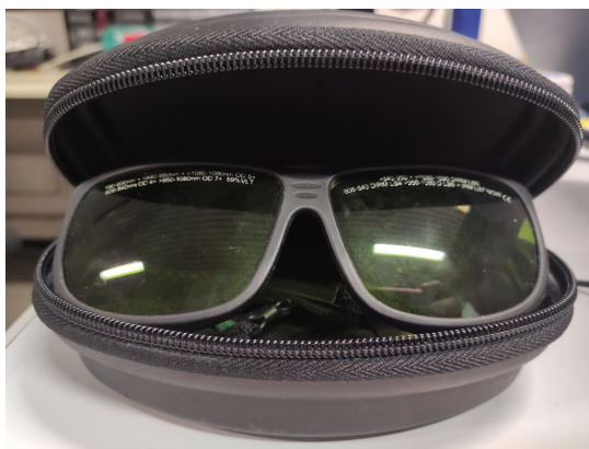
Figure 3.11: Global Laser safety glasses; this model blocks light within the wavelength range of \sim 840 \div 1090 nm.
