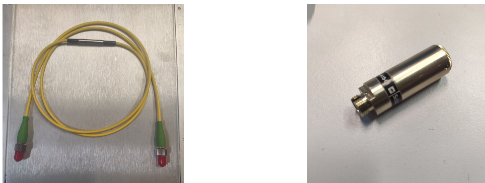
Figure 3.6: One of the three Thorlabs fibers used (left), specifically the one terminated with the collimator (right).
