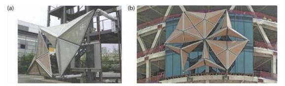
Figure 75 (a) A full-scale prototype of the mashrabiya undergoing mechanical testing at Yuanda's facilities in Shenyang (Aeadas Architects Ltd) and (b) the onsite benchmark for six mashrabiyas. Source: www.glassonweb.com
