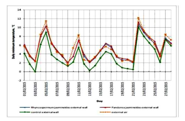
Figure 29 Daily minimum surface temperature of the external plaster of the three walls exposed to solar radiation and daily maximum external air temperature measured
