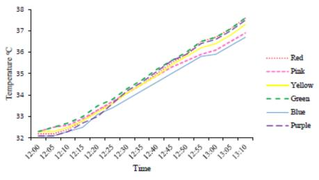
Figure 52 Temperature rise of the liquid enclosed in a colored acrylic box
