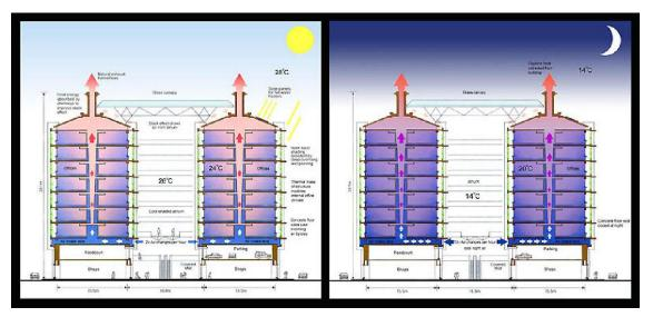
Figure 72 Eastgate Centre ventilation system Source mickpearce.com/Eastgate.
