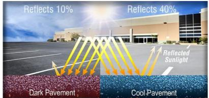
Figure 5 Diagram illustrating how Cool Pavement coating will increase solar reflectivity. Source: www.geographyrealm.com/can-painting-city-streets-reduce-urban-heat-island-effect/
