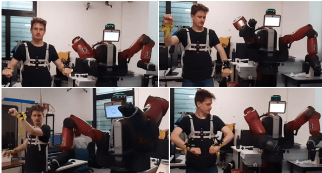
Figure 4.4: Dual-arm Cartesian teleoperation.
