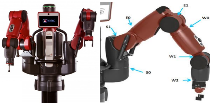
Figure 2.5: Baxter Humanoid Robot (Left) and Baxter's Arm and Joint Designations (Right).
