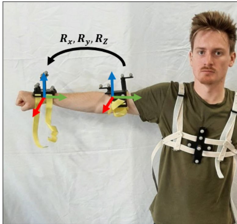
Figure 3.5: Elbow calibration of a single arm. The operator keeps the calibration position to compute any possible misalignment between the elbow and the wrist reference frame.
