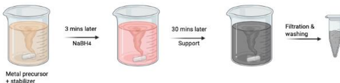
Figure 10. Scheme of Sol-Immobilization method to synthesize supported metal nanoparticles.
