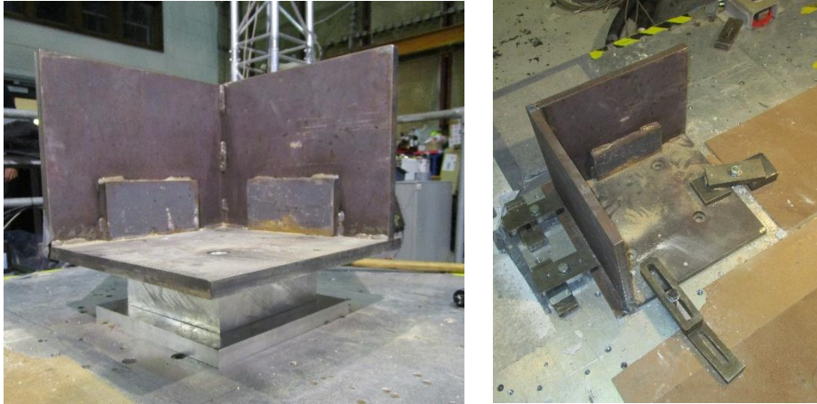
Figure 30: Corner steel plates.
