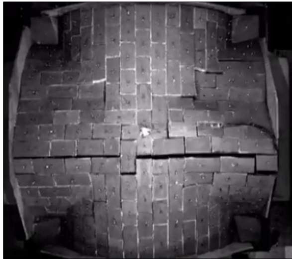
Figure 53: Crack opening leading to collapse in test 52.
