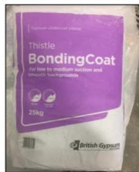
Figure 29: Bonding Coat by British Gypsum used in the experimental campaign.
